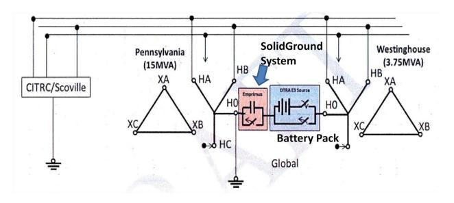
Figure 3 - Idaho National Laboratory Experimental Configuration for testing the Neutral Blocking System
