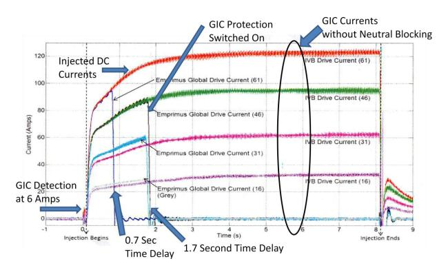
Figure 4 -  $SolidGround^{TM}$  Neutral Blocking Live Grid Test Results
