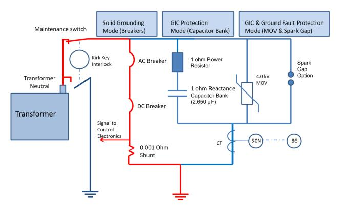
Figure 2 - Diagram of the SolidGround Transformer Neutral Blocking System
